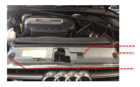
3 Disconnect the bonnet latch cable and crash sensor. Remove the crash sensor wiring harness from the radiator assembly shroud at the 3 x mounting points (2 of 3 points are pictured) and gently place in the engine bay, out of the work area.
