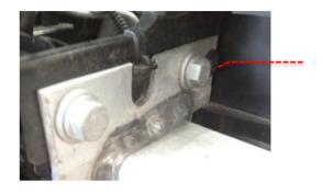
Remove the T30 bolt at each upper corner of the radiator assembly shroud (2 in total).
