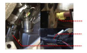
Disconnect the air temperature sensor under the crash bar. Disconnect the sensor harness from the 5 x harness routing clips and place the harness/connector into the engine bay, out of the work area.
