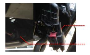
11 Remove the 2 x T30 bolts at the top corner of the bumper cover. Remove the T30 bolt inside the back of the bumper cover, holding the cover to the chassis. Repeat on the opposite side of the vehicle.
