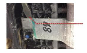
Lean the radiator/intercooler towards the engine and remove the yellow hanger brackets. Note the orientation of the clips for reinstallation. Place outside of the work area. Carefully press down on the tabs that lock the radiator to the top of the intercooler. Using a screwdriver against the metal radiator/intercooler seams, apply light pressure to free the intercooler from the radiator. Note: be careful, the radiator is easily damaged if excessive force is used.
